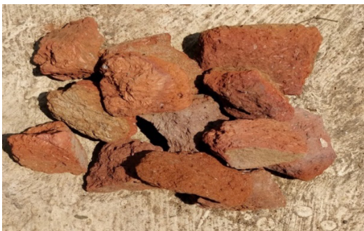
Fig. 2. Over burnt clay brickbats used as contact media in the experimental setup
