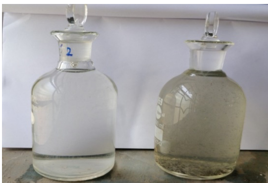
Fig. 11. Sewage sample before treatment (right) and after treatment sample (left) at 3.0 m depth and 2.5 l/hr rate of flow
